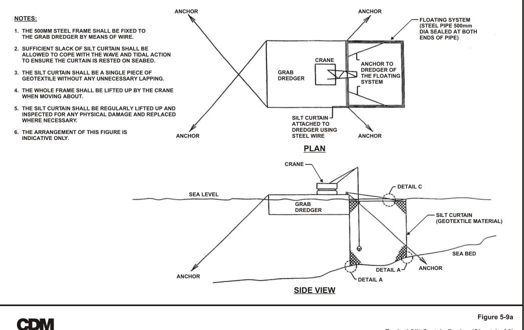
Typical Silt Curtain Design (Sheet 1 of 3)
